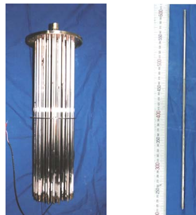
Fig.3 Mold bundle after casting (left) and U-Zr slug after mold removal (right)
