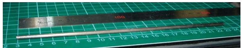
Fig.4 Cast U-20wt%Pu-10wt%Zr alloy slug (200mm in length) fabricated by injection casting method. Smooth and metallic surface in the whole length can be seen.
