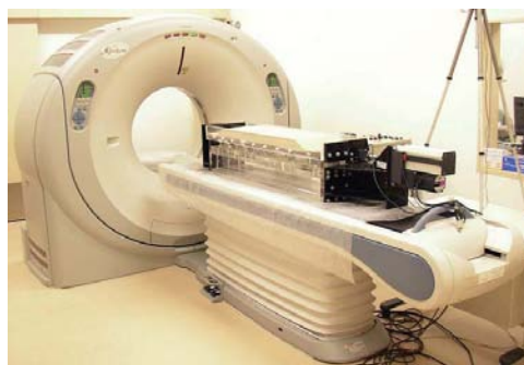
Helical X-ray CT scanner and experimental apparatus used for fault modeling.
