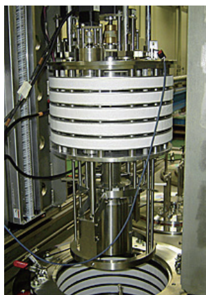
Fig.4 The electrorefining apparatus (left) and cathode deposit (right)
