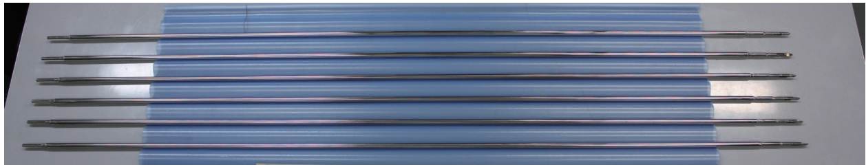
Fig. 1 Metal fuel pins ( \phi 8 \times 600\text{mm} ) for an irradiation test in the experimental fast reactor Joyo
