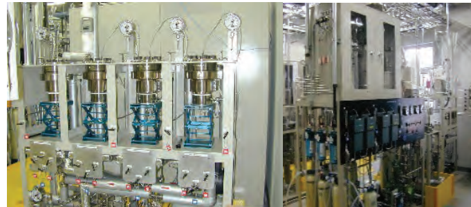
High temperature and high pressure loop system for corrosion evaluation
