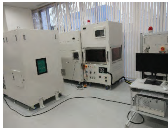
Evaluation equipment of current-voltage and switching characteristics of power semiconductor devices
