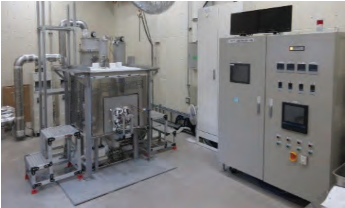
Vitrification experiments using small-scale glass melter
