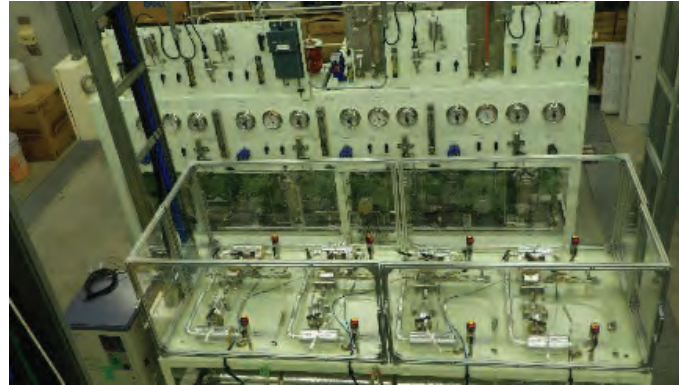
High flow velocity and high temperature loop system for corrosion evaluation
