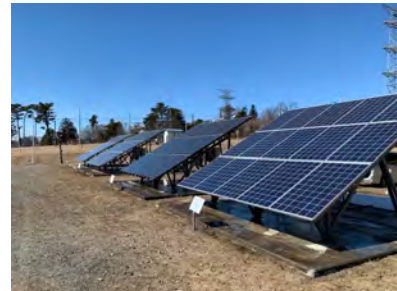
Performance measurements of PV systems composed of various PV technologies at the Akagi Testing Center
