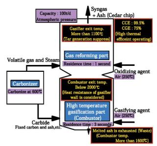
Fig.2 Schematic of carbonization and gasification system
