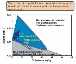
Fig.5 Operating condition range for high thermal efficiency and stability when volatile ratio is changed.
