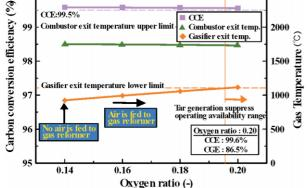
Fig.3 Gasification performance in carbonization and gasification system (Cedar chip, Combustor oxygen ratio = 0.56. Air is fed to gas reformer)
