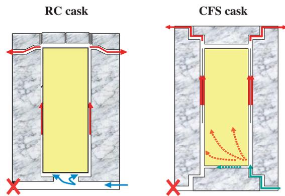
**Fig.4** Flow patterns under 50% blockage of the inlet
