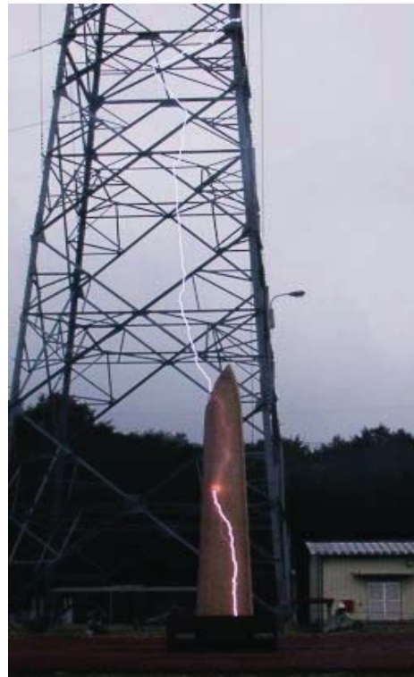
Fig.2 Lightning discharge on wind turbine blade model
