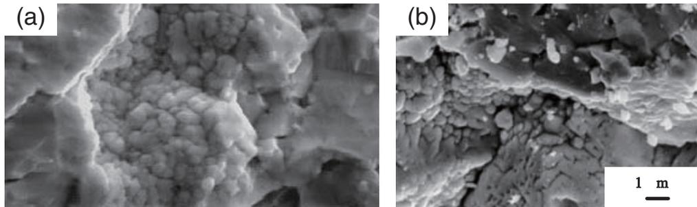
**Fig.2** SEM images of (a)(U,Gd)O<sub>2</sub> fuel of 53 MWd/kgU, 880°C, and (b)UO<sub>2</sub> fuel of 51 MWd/kgU, 880°C
