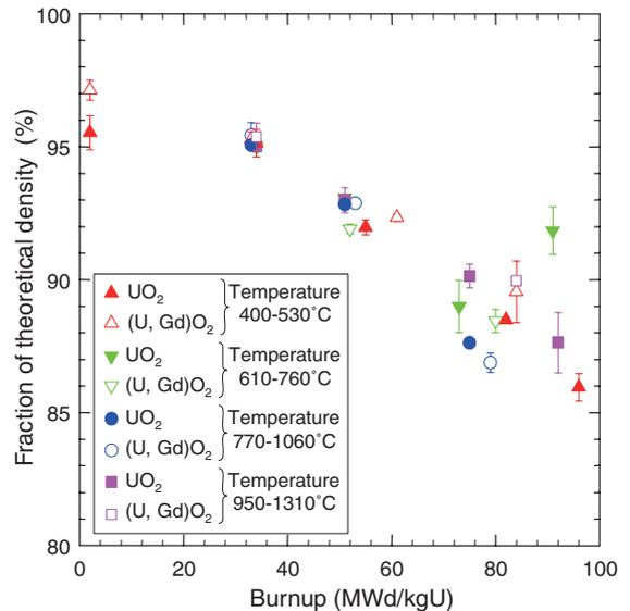
**Fig.4** Densities of UO<sub>2</sub> and (U, Gd)O<sub>2</sub> fuels as a function of burnup
