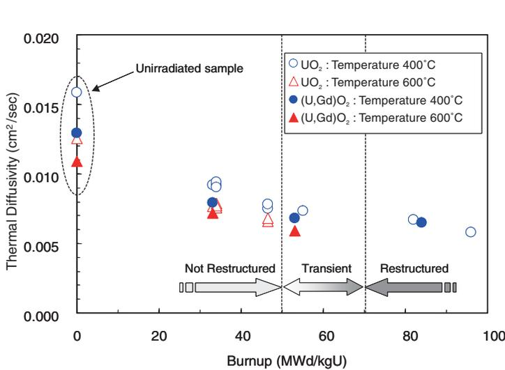
**Fig.3** Thermal diffusivities of UO<sub>2</sub> and (U, Gd)O<sub>2</sub> fuels as a function of burnup (No-adjustment of porosity)
