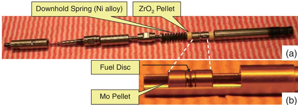
**Fig. 1** Mounting of irradiation rig. (a) Single parts, (b) fuel disc in centering ring between Mo pellets
