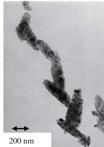
**Fig.2** TEM micrograph of CGO by a large scale bath with a capacity of 65 kg/batch
