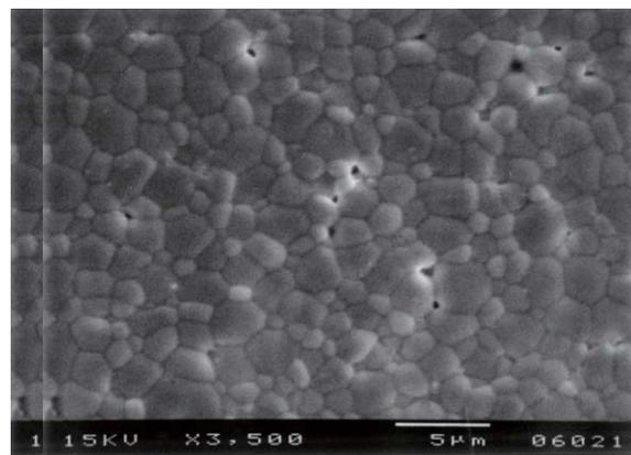
**Fig.4** Scanning electron microscopy (SEM) micrograph of CGO electrolyte on the porous anode in IT- SOFCs
