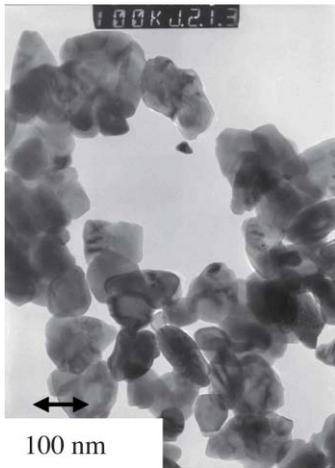
**Fig.1** Transmission Electron Microscopy (TEM) micrograph of CGO by a small scale bath with a capacity of 0.1 kg/batch
