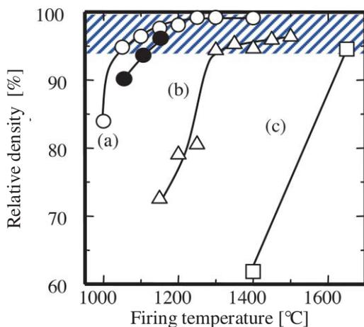
**Fig.3** Relative densities of CGO synthesized by various methods, as a function of firing temperature
