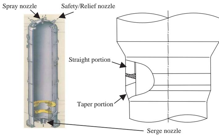
**Fig.1** Pressurizer's dissimilar metal weld
