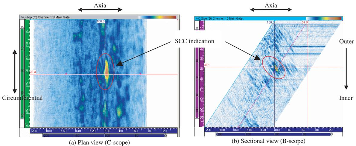
**Fig.3** Example of UT examination data: axial scanning from nozzle side to safe-end (Circumferential 18% through wall depth SCC in Serge nozzle)
