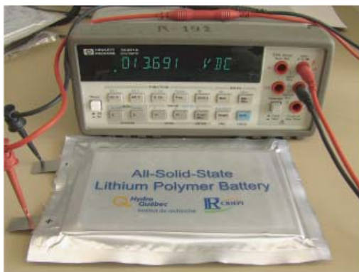
Fig.3 Operated 4-stack cell (13.69 V, 13x8cm flat-type. No additional pressure from outside)
