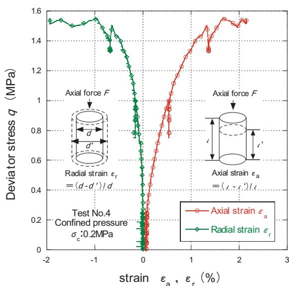
**Fig.3** Relationship between stress and strain
