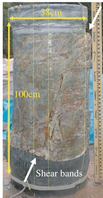
**Fig.2** Specimen retrieved after tests
