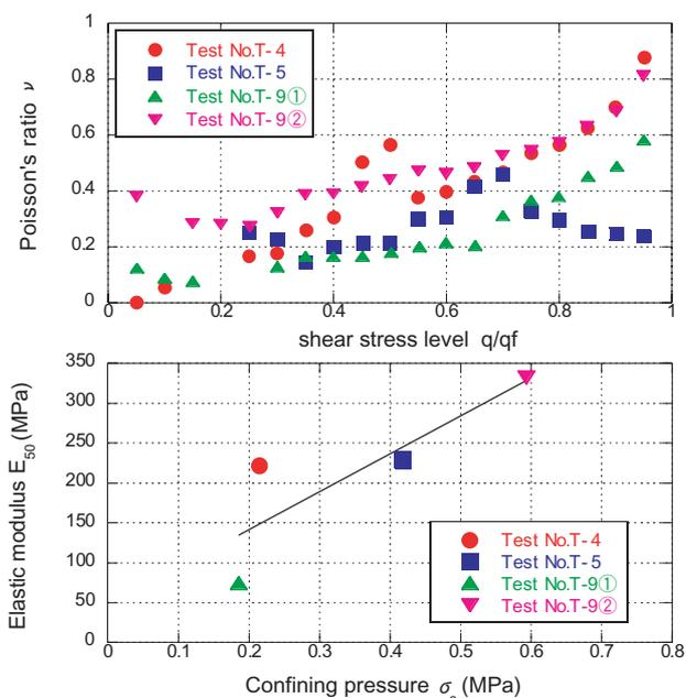
**Fig.4** Mechanical properties of the site
