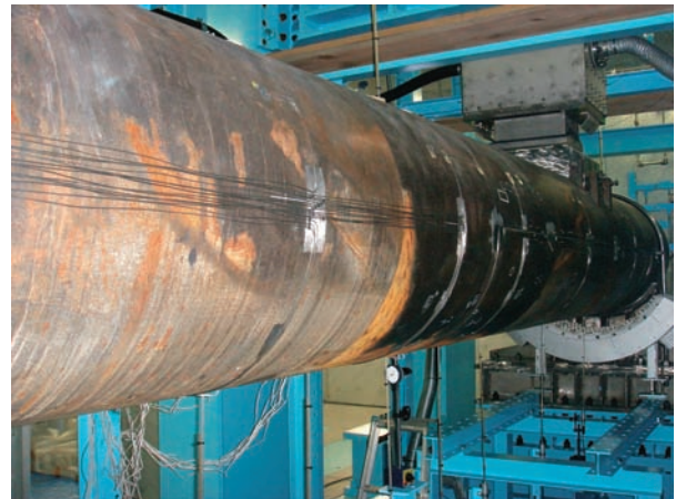
(b) Installation of welded pipe to test facility BIPress
