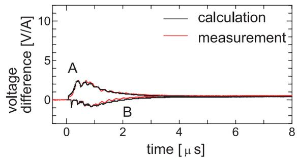
(d) voltage difference between the grounding grid and the control wire
