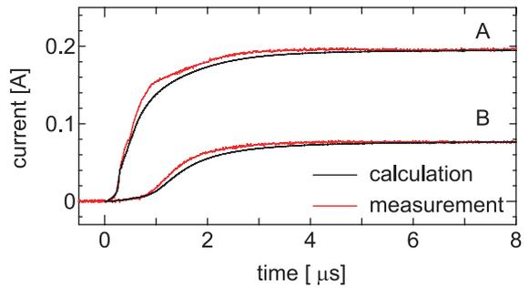
(d) Current propagating through the grounding grid
