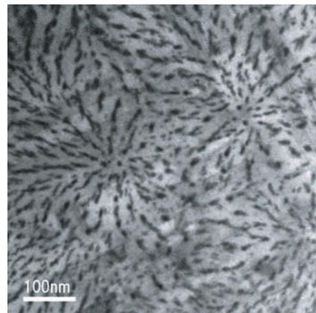
**Fig.4** Plan-view TEM image of the particular structure of  $\text{YBa}_2\text{Cu}_3\text{O}_y$  film contained  $\text{BaZrO}_3$ .
