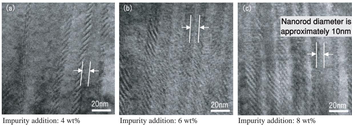
**Fig.2** Cross-sectional TEM images of YBCO superconducting films with various impurity amounts. Nanorods indicate the inclined or vertical stripes gone through from bottom to top sides. It is found that the number density of nanorods increases without changing diameter in various impurity additions.
