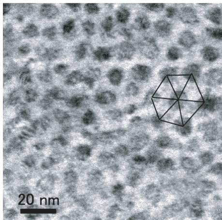
**Fig.3** Plan-view TEM image of  $\text{YBa}_2\text{Cu}_3\text{O}_y$  film contained 10 wt%  $\text{BaZrO}_3$ .
