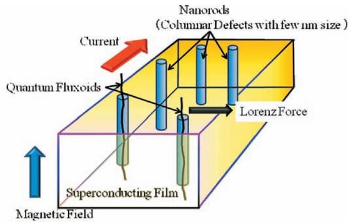
**Fig.1** Conceptual configuration of nanorods as pinning centers
