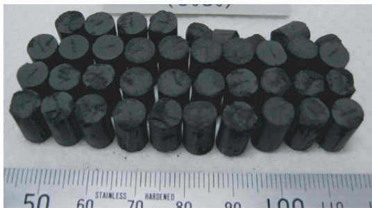
Fig. 2 Oxide pellets with 32% of porosity prepared by pretreatment process: UO 2 containing 1 wt% of each simulated FP (Ce, Nd, Sm, Sr, Zr, Mo and Pd).
