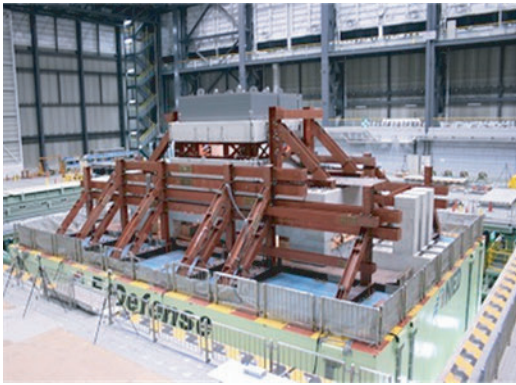
Fig.1 Test specimen of seismically isolated structure and lead rubber bearing (LRB)
