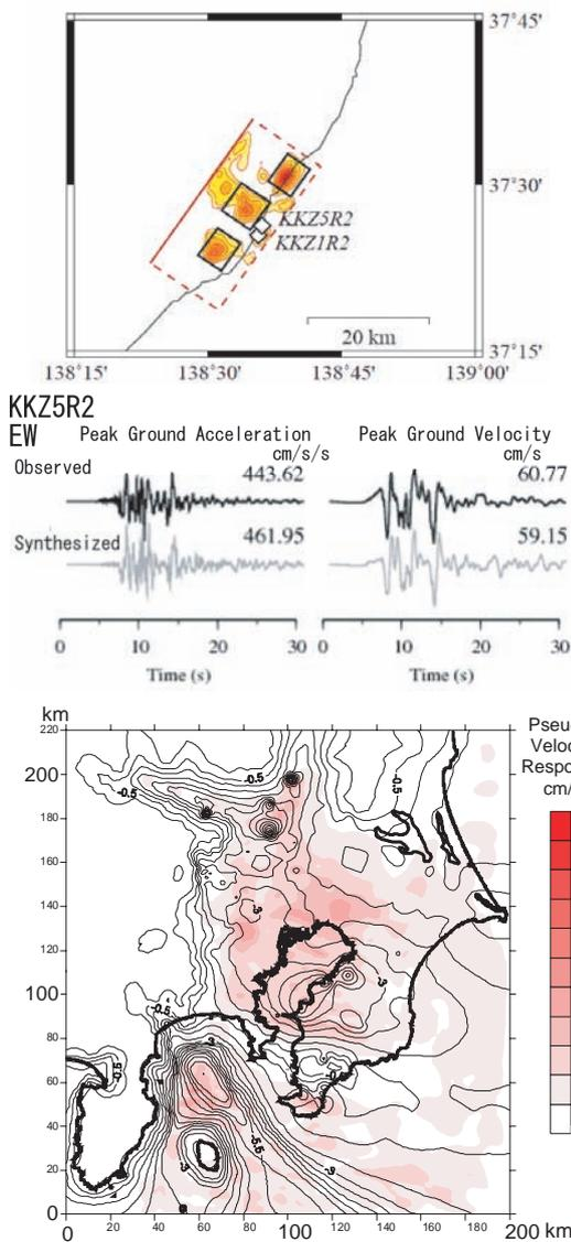
Fig.3 An example of the pseudo-velocity response distribution at the period of 8 sec. in the Kanto Plain (h=0.01). Contour lines represent the depth of the seismic basement (unit: km).
