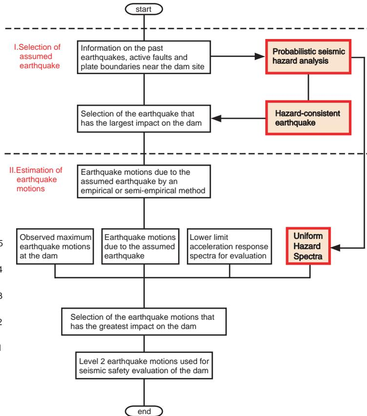
Fig.4 An example of the introduction of the probabilistic approach into the MLIT guidelines for seismic safety evaluation of dams (red boxes).
