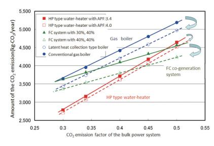
Fig. 2 Comparison of CO<sub>2</sub> emissions from residential houses installed with high efficiency water-heater systems with consideration given to residential demands.
