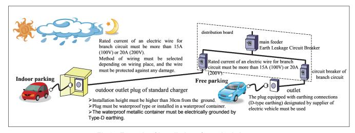
Fig.3 Example of installation of standard charger
