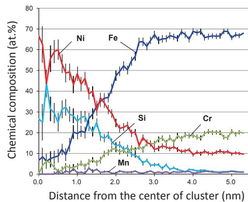
**Fig. 3 Chemical composition of region where solute atoms concentrate in irradiated stainless steel**
