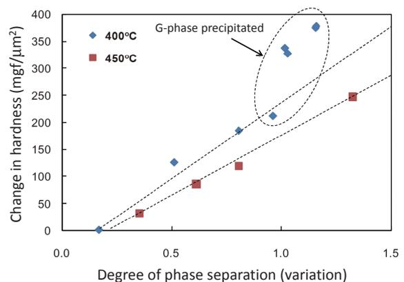
**Fig. 5 Correlation between change in hardness and phase separation**
