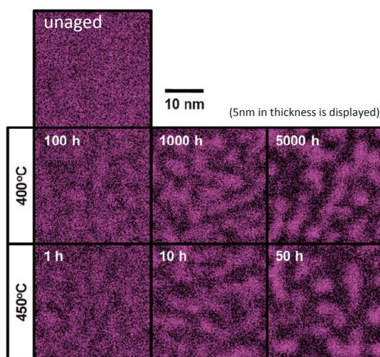
**Fig. 4 Phase separation in ferrite phase of duplex stainless steels**
