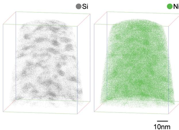
**Fig. 2 Distribution of silicon (Si) and nickel (Ni) atoms in irradiated stainless steel**
