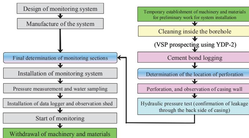
**Fig. 1 Build process of monitoring system**
