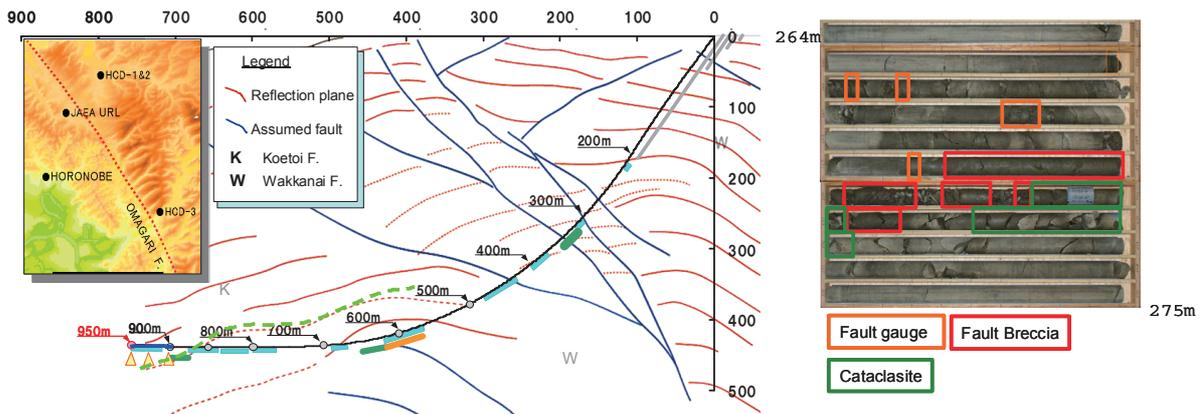
**Fig. 2 Outline of the directional drilling (Left: drilling trace, Right: Rock core sample of fault zone)**
