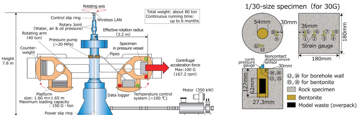
**Fig. 3 Acceleration test of the near field behavior by centrifuge (Upper left: Centrifuge, Upper right: Model of near field, Lower right: Picture of the near field model taken by X ray CT)**
