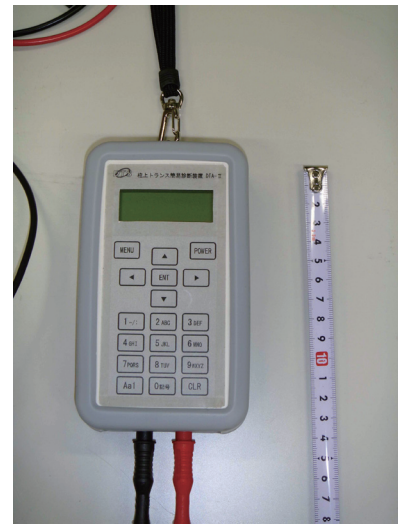
Fig. 2 Portable layer short-circuit checker of a pole transformer
