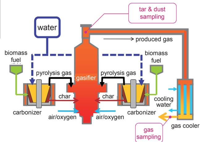
**Fig. 2 Flow diagram of biomass carbonizing gasification test facility**
