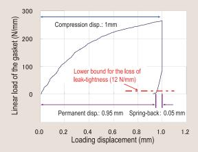
Fig. 4: Ageing effect on the load-deflection curve of the metal gasket after 60 years of usage
