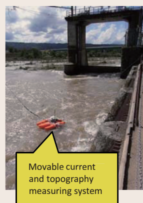
Fig. 4: Movable current and topography measuring system
