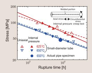
Fig. 3: Results of creep test of 9Cr steel welded joints
