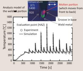
Fig. 2: Welding simulation of 9Cr steel
