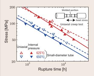
Fig. 4: Results of creep test of 12Cr steel welded joints
