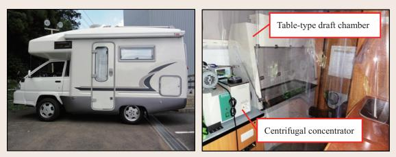
Fig. 1: Prototype vehicle for PCB analysis (left) and analytical instruments inside the vehicle (right)
