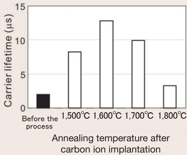
Fig. 1: Changes in the carrier lifetimes of SiC epilayers before and after the carbon ion implantation and annealing process with different annealing temperatures
