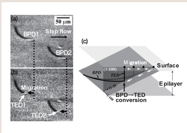
Fig. 2: Conversion of BPDs to TEDs by high-temperature annealing
