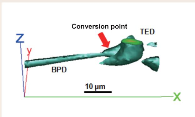
Fig. 3: Three-dimensional synchrotron X-ray topography image taken for a position of BPD-TED conversion
