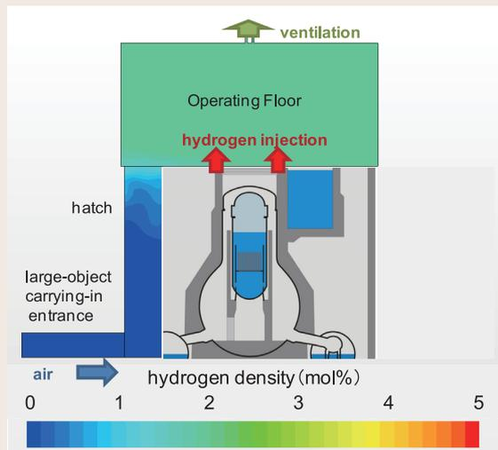
Fig. 4: Calculation on hydrogen behavior in BWR building
