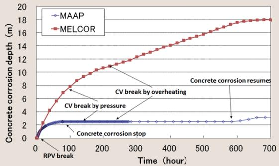
Fig. 2: Comparison between codes of the concrete corrosion depth in a containment vessel (CV) about the accident sequence "large rupture LOCA + feed water failure" in a PWR representation plant
