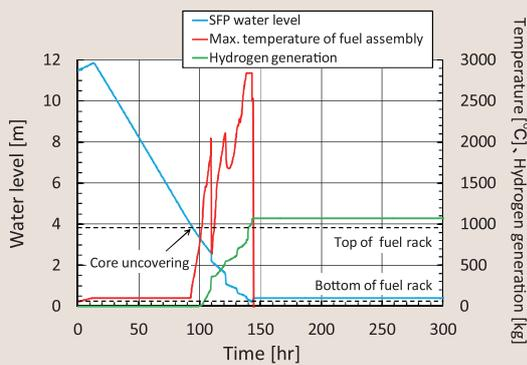
Fig. 3: Evaluation of spent fuel pool in a loss-of-coolant accident due to station power outage
