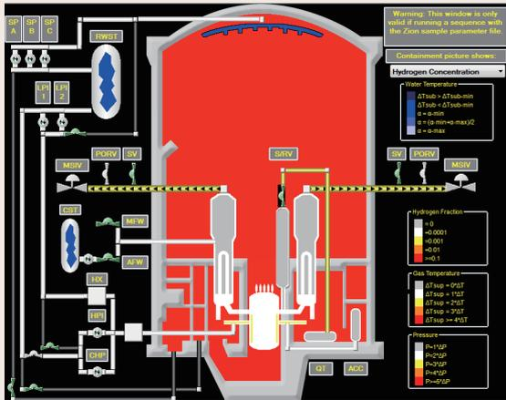
Fig. 1: Analytical model and graphics of calculation results for a typical PWR plant in the MAAP code
