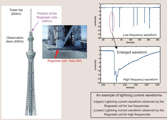
Fig. 2: Lightning current observation system installed on the TOKYO SKYTREE and an example of observed lightning current waveforms
