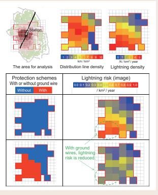
Fig. 1: Difference of lightning risks of high-voltage distribution lines with different lightning protection schemes
