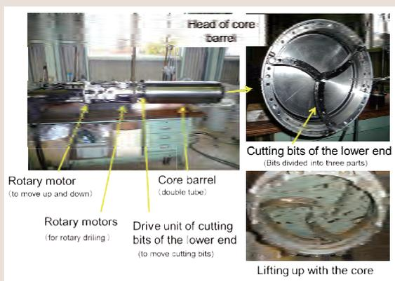
Fig. 3: Sampling equipment using a large-scale rotary tube
