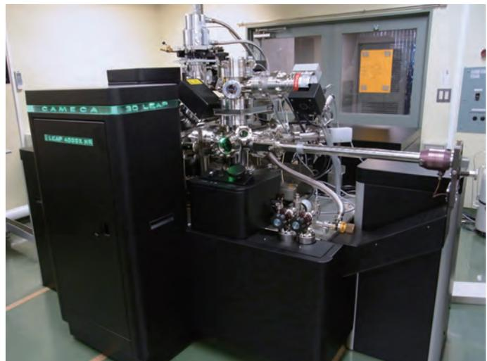
Appearance of three dimensional atom probe (front view)
