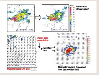
Fig. 3: Improving the accuracy of short-range rainfall forecasting using NCAR VDRAS
