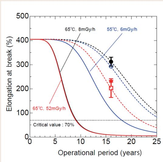
Fig. 1: Comparison of aging trends in service-used cables and aging prediction by the ACA project
