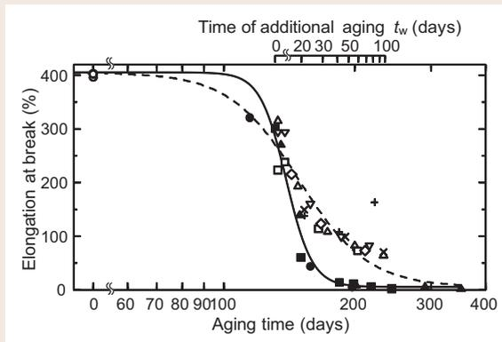
Fig. 4: Comparison of the mechanical aging trend during the wear-out test to that predicted based on the ACA project result
