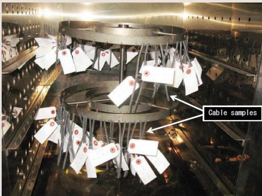
Fig. 3: A thermostatic oven during the wear-out additional aging test
