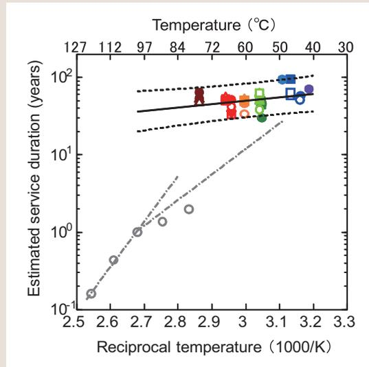
Fig. 2: Service duration estimated for cables used in nuclear power plants and their temperature in an Arrhenius plot
