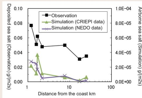
(b) Comparison with observation data (measured values using ACM sensors by TEPCO)
