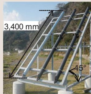
(b) Photo of diagonal braces arranged at a testing field.
