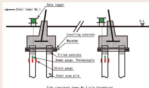
Fig. 3: Dynamic observation equipment of steel tower pile foundation
