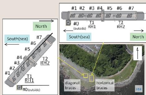
(a) Schematic diagrams of ACM sensors arranged in horizontal and diagonal braces arranged at Yokosuka coastal testing field.
