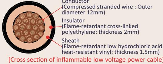
[Cross section of inflammable low voltage power cable]
