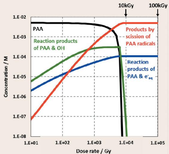
Fig. 4: Results of radiation chemical simulation of PAA solution (PAA 500 ppm, 300°C, neutral pH)
