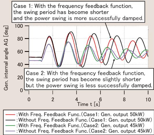
Fig. 2: Results of testing using CRIEPI's Power System Simulator
