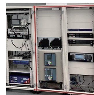
Verification equipment of IEC 61850-compliant substation system
