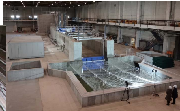
The whole view of Tsunami physical simulator And breakwater overflows experimentation
