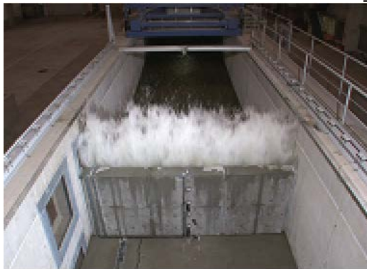
The whole view of Tsunami physical simulator And breakwater overflows experimentation
