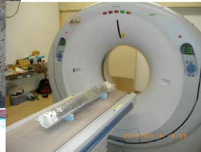
A look of investigation of active fault, and Sample analysis with X-ray computed tomography scanner
