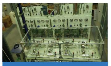
High flow velocity and high temperature loop system for corrosion evaluation
