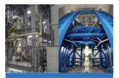
Test facility for three-dimensional thermal hydraulics in light-water reactors (SIRIUS-3D)
