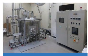
Vitrification experiments using small-scale glass melter
