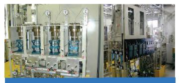
High temperature and high pressure loop system for corrosion evaluation
