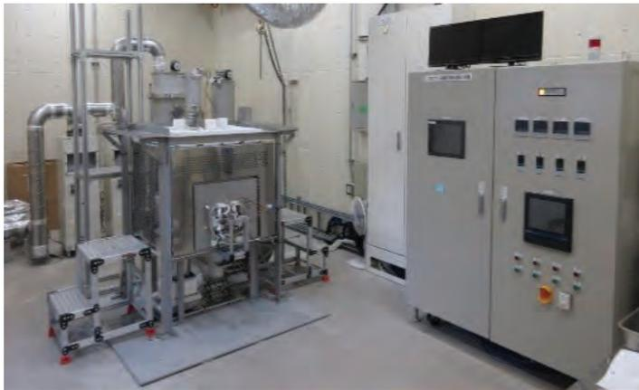
Vitrification experiments using small-scale glass melter
