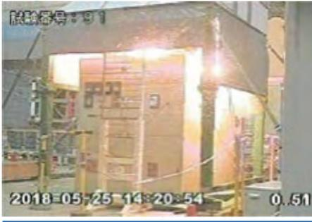
**HEAF (Arc internal Test on the electrical equipment)**
