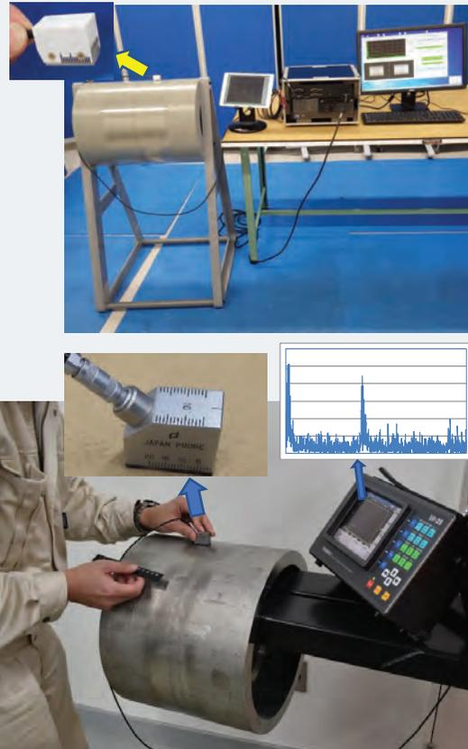
Virtual UT (Ultrasonic Testing) system
