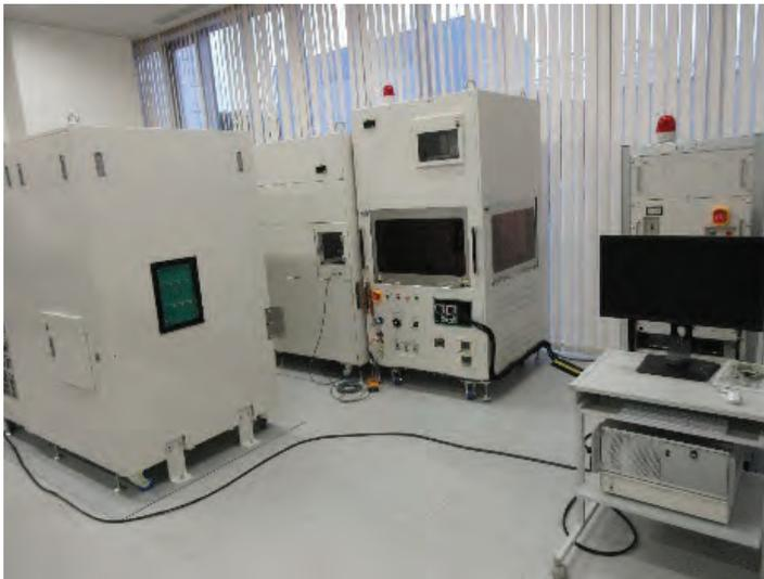
Evaluation equipment of current-voltage and switching characteristics of power semiconductor devices
